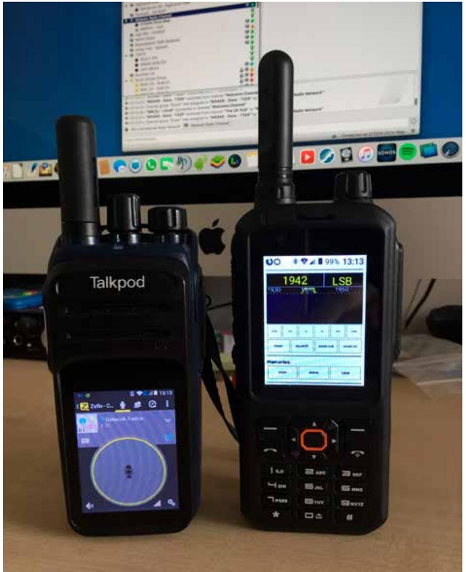
**Fig 1: A Talkpod N58 running Zello & an Inrico T320 monitoring a Topband WebSDR. The desktop behind is running IRN.**
